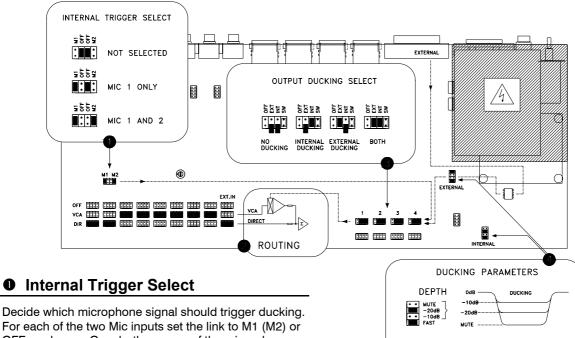
For each of the two Mic inputs set the link to M1 (M2) or OFF as shown. One, both or none of the microphones can trigger ducking.
