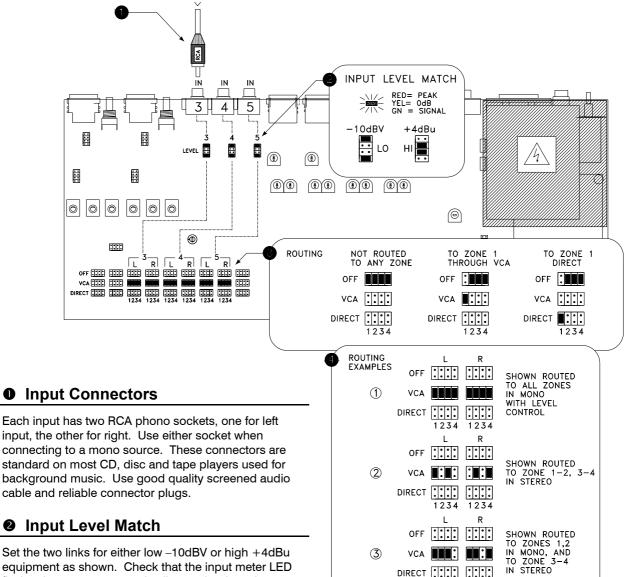
Set the two links for either low -10dBV or high +4dBu equipment as shown. Check that the input meter LED flashes between green and yellow on loud music. Reposition the links if the meter reads too low or if the red peak indicator flashes.
